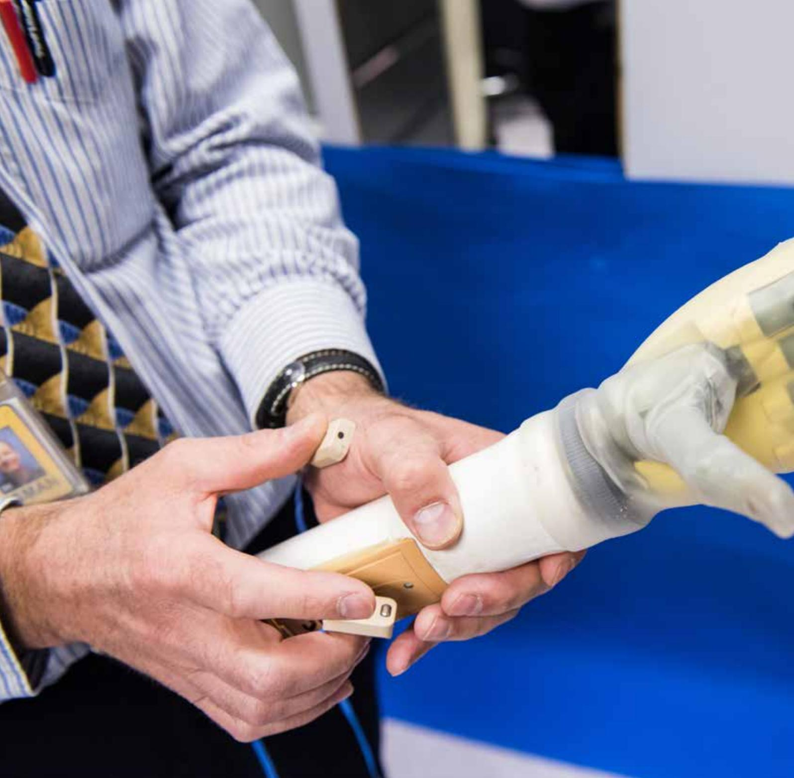
thumb movement would fire a signal. Polymer would pick up that signal and convert it to an electronic signal, which would wirelessly control a motor to move the thumb on the prosthesis.
